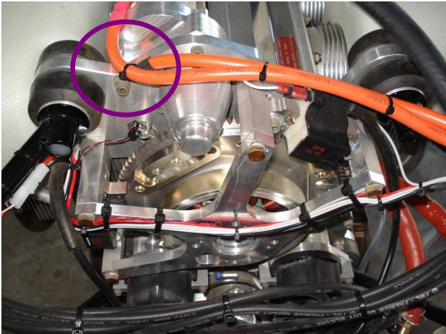
Figure 1: Cable to Engine Backing Plate
